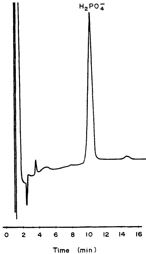
FIGURE 1: Chromatogram of a standard solution of dihydrogen phosphate (20 \mu\text{g}/\text{ml} ).
